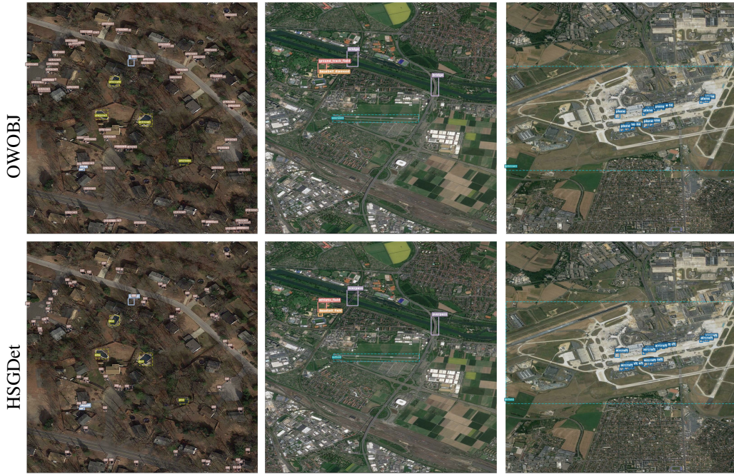
Figure 3. Comparison between OWOBJ and HSGDet on DOTA-v2. OWOBJ detects the unseen objects without semantic grounding, whereas HSGDet detect the unseen object with proper class labels.
